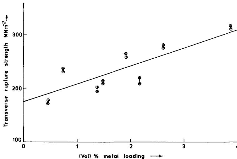
Figure 6 Transverse rupture strength of PVC-copper composite as a function of vol % metal loading.
