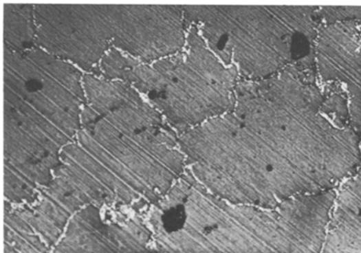
Figure 4 Segregated network of copper in PVC matrix in compression-moulded briquette,  $\times 300$ .
