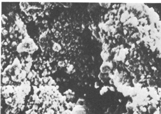
Figure 2 SEM showing dispersion of copper particles on PVC surface,  $\times 5000$ .
