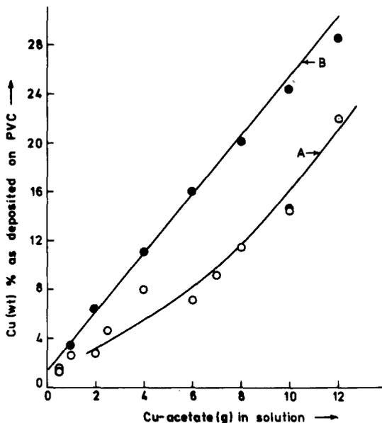
Figure 3 Actual (A) and theoretical (B) amount of copper deposited as a function of amount of copper acetate solution.
