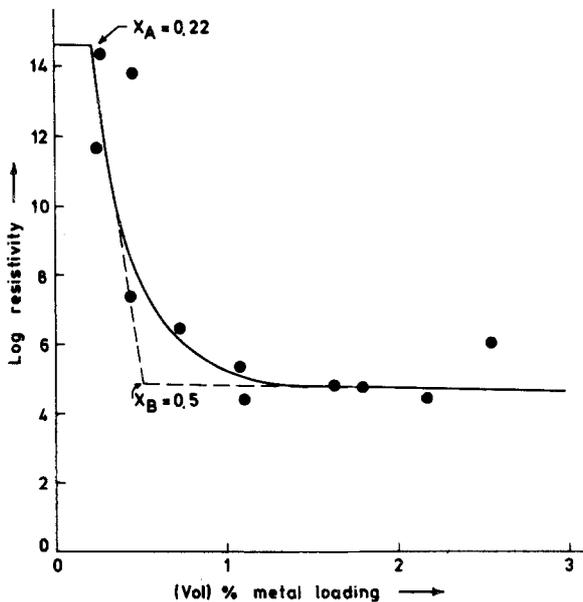
Figure 5 Electrical resistivity as a function of metal loading.
