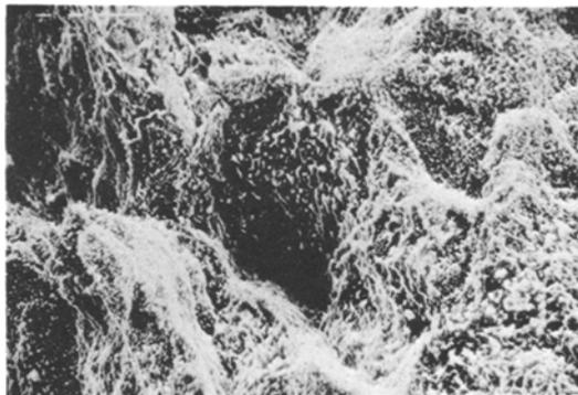
Figure 7 SEM fractograph of PVC-Cu composites showing interparticle fracture and fine flow lines.
