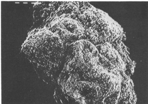
Figure 1 Scanning electron micrograph of PVC particles showing deposited copper on the surface,  $\times 650$ .
